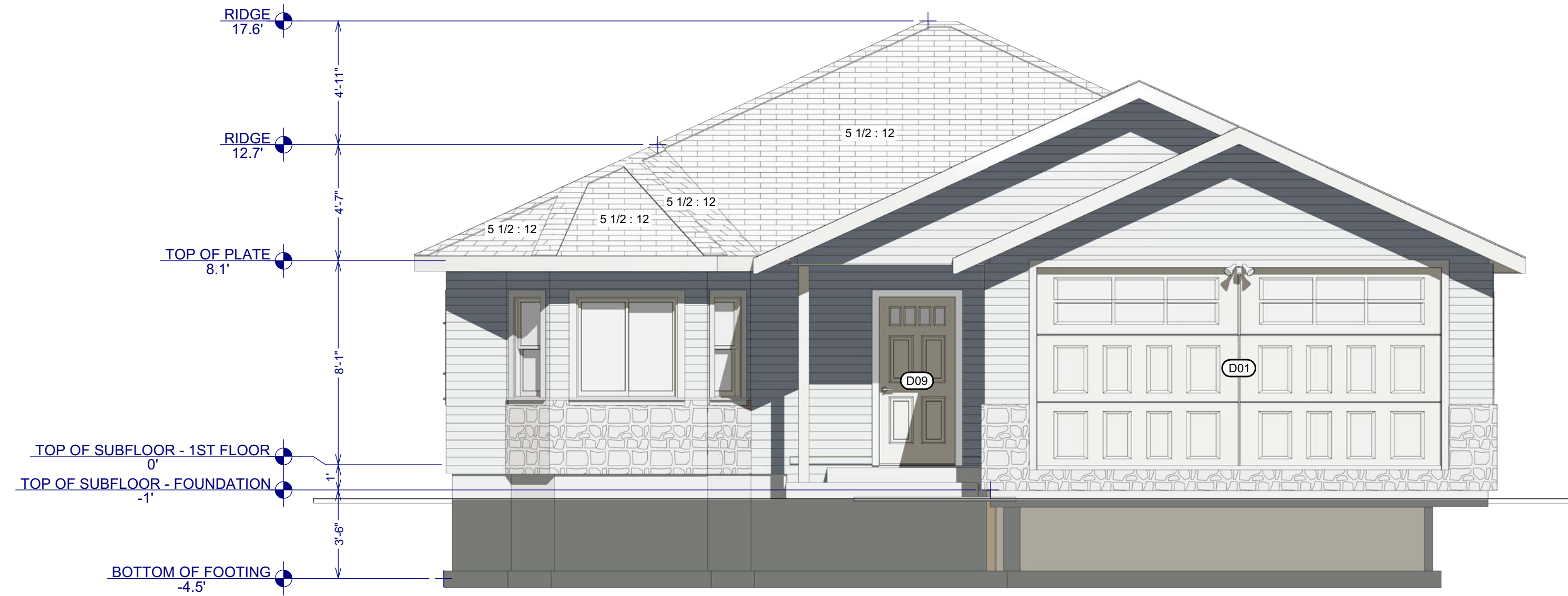
Exterior Elevation Front 1/4 in = 1 ft
