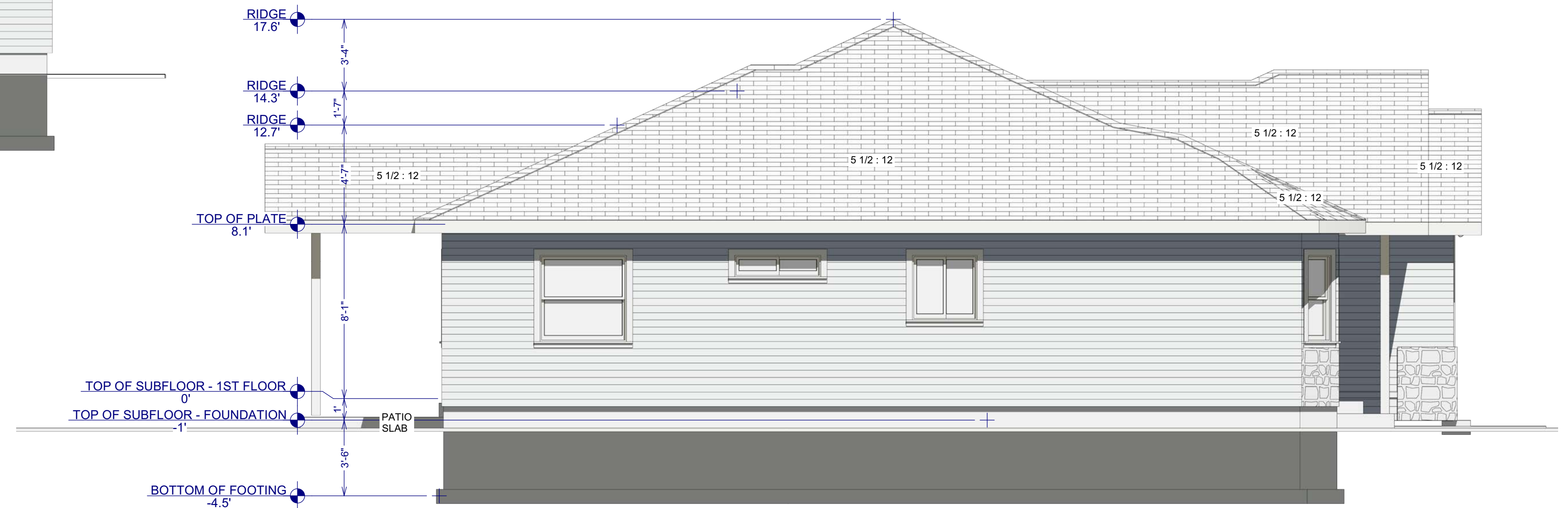
Exterior Elevation Left 1/4 in = 1 ft
