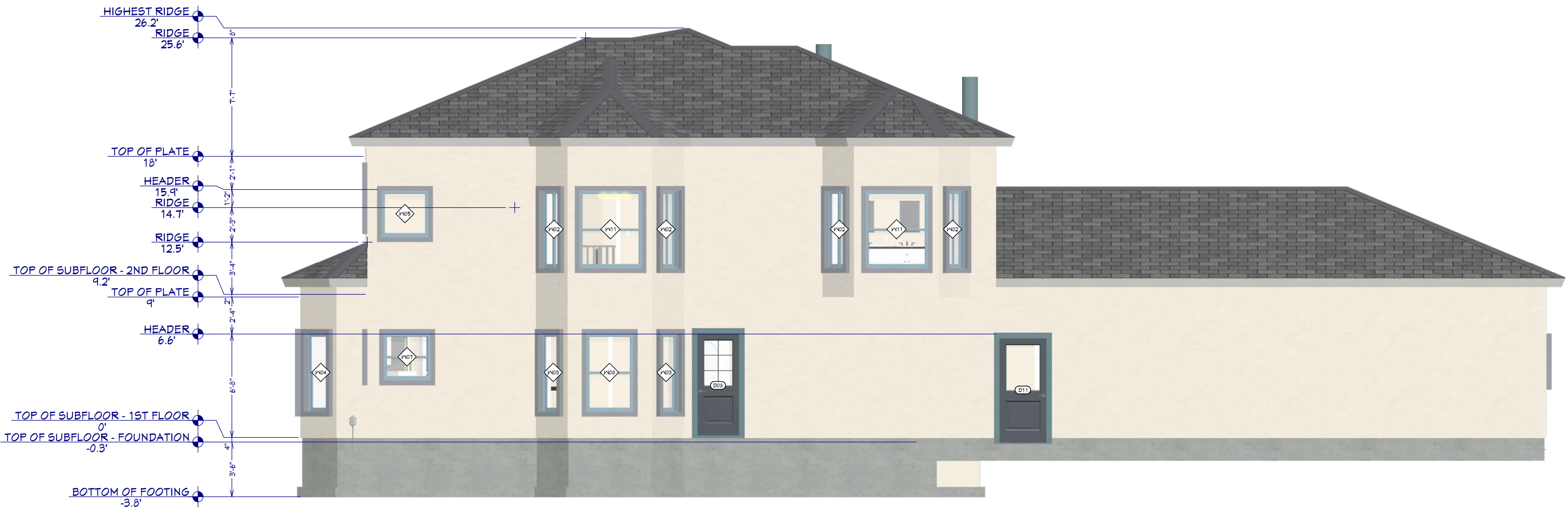
Exterior Elevation Back Scale: 3/16" = 1'-0"
