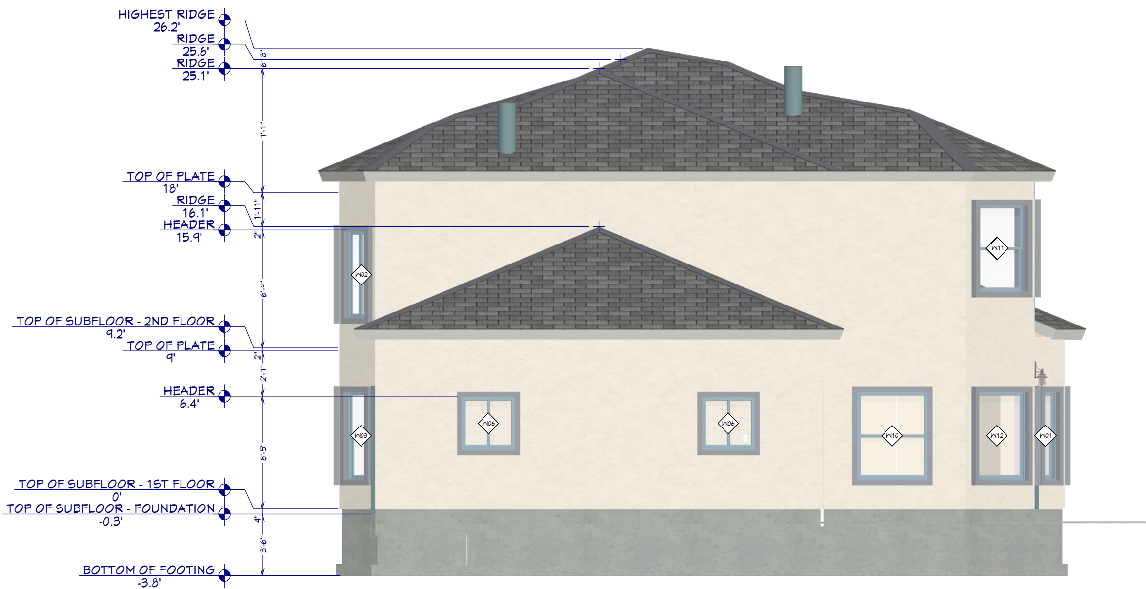
Exterior Elevation Left Scale: 3/16" = 1'-0"
